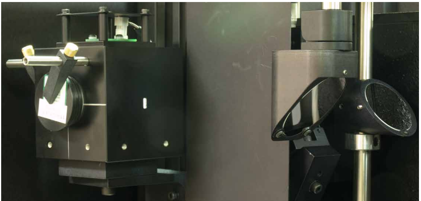
Flipping the mirror on the right lets the probe beam enter the integrating sphere on the left. The sphere is designed for maximum reflectance measurement accuracy on solar cells.
